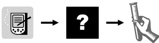
Figure 12 Schematic illustrating the desired behavior of an automated chemical reactor. The user enters the desired particle properties, the “black-box reactor then evaluates multiple reaction conditions until it identifies an appropriate set that yield particles with the desired properties; the reactor then continues to produce particles with these properties until instructed to stop.
